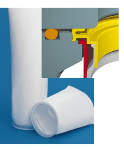
Now, applications requiring polypropylene or polyester felt filter bags can take advantage of the all-welded construction afforded by patented SENTINEL® Filter Bags. These bags, made from silicone-free materials, feature super-strong welded construction rather than sewn seams. This construction ensures that nothing bypasses the process media through holes in sewn fabric.
