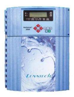
The process photometer **Testomat 2000® Polymer** is a robust wet-chemical online monitor for monitoring the polyacrylate content from 0 to 50 mg/l (ppm) (with the factor set to 1.00) using the photometric analysis principle.
