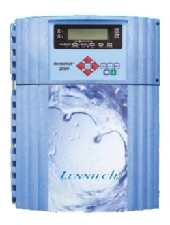
The **Testomat 2000® CrVI** process photometer is a robust wet-chemical online monitor used to monitor chromate content (CrO<sub>4</sub><sup>2</sup>) within the range of 0 to 2.0 mg/l, or hexavalent chromium (CrVI) within the range of 0 to 1.0 mg/l. The device operates with a photometric analysis principle on the basis of the DIN 38405 standard.
