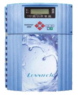
Concentrations of oxidising agents, such as chlorine, chlorine dioxide or ozone, above TVO-approved (German drinking water ordinance) limit values have a detrimental effect on the dye contained in Testomat 2000® reagents. Exact determination of the water hardness is therefore no longer guaranteed, and the Testomat instrument displays the error message 'measuring fault analysis' (MST analysis). To execute the measurement correctly, a reducing agent must be added.
