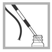
**10.** When the timer expires, turn off the UV lamp. Remove the UV lamp from the sample.
