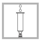
**2.** Use a syringe to push at least 50 mL of sample through a 0.22-micron filter membrane apparatus.
