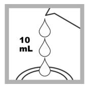
**3. Prepare the blank**: Fill a sample cell to the 10-mL mark with filtered sample from step 2.
