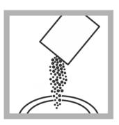
**12.** Add the contents of one PhosVer 3 Phosphate Reagent Powder Pillow to both the blank and the prepared sample.
