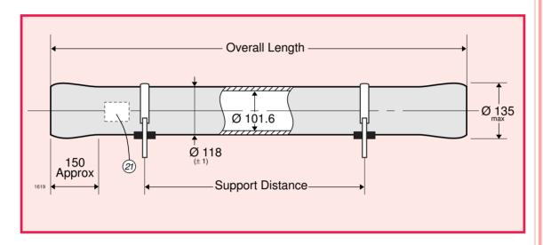
Body of vessel is manufactured completely from glass reinforced epoxy resins.
