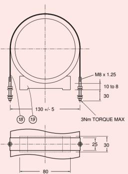
Tighten all bolts/nuts to 50% of the maximum torque figure.
