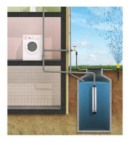
Submersible pump with asyncronous single phase motor, stainless steel pump body and stainless steel motor shaft. SUB 6S Plus has a double mechanical seal increasing the shaft resistence to stress due to the pump working.
