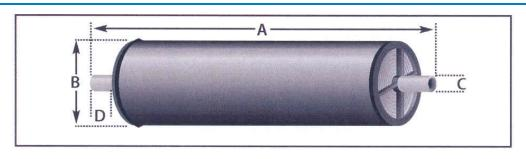
С Model D Weight Part Numbers inches (mm) inches (mm) inches (mm) lbs (kg) Interconnector O-ring Brine Seal 0035458 0035702 40 (1,016) 0.75 (19.0) 1.0 (25.4) 10 (4.5) 4040-FR 4 (101.6) 0035267
