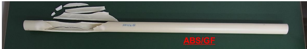
Permeate core tube collapse and mechanical failure.
