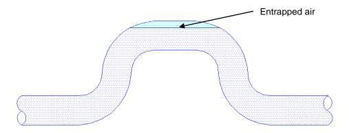
Should pipe-work layout constraints make it impossible to avoid such instances, provision for the automatic venting of entrapped air should be made at the uppermost section of the pipe-work.
