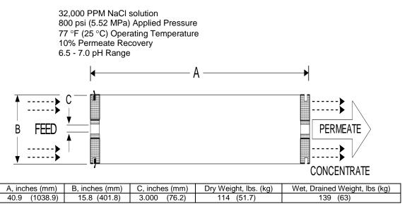
Notice: Permeate flow for individual elements may vary + 15 /-15 percent. Membrane active area may vary +/-4%. All membrane elements are supplied with a brine seal, interconnector, and o-rings. Elements are enclosed in a sealed polyethylene bag containing less than 1.0% sodium meta-bisulfite solution, and then packaged in a cardboard box.
