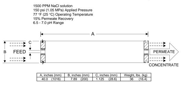
Notice: Permeate flow for individual elements may vary + or - 15 percent. Membrane active area may vary +/-4%. Element weight may vary. All membrane elements are supplied with a brine seal, interconnector, and o-rings. Elements are enclosed in a sealed polyethylene bag containing less than 1.0% sodium meta-bisulfite solution, and then packaged in a cardboard box.
