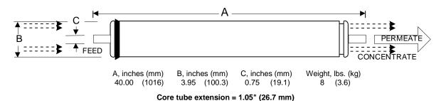
**Notice:** Permeate flow for individual elements may vary -20 or +25 percent. All membrane elements are supplied with a brine seal, interconnector, and o-rings. Elements are enclosed in a sealed polyethylene bag containing less than 1.0% sodium meta-bisulfite solution, and then packaged in a cardboard box.
