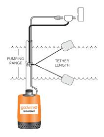
Pumping range determined by tether length according to the following guide.
