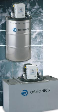
The WasteWizard system is a compact, fully-integrated system for point-ofuse recycling. The system comes complete with its own fluid transfer system that automatically exchanges the dirty cleaner from the washer with recycled cleaner. The WasteWizard system sits on a standard 55 gallon (200 L) drum or optional 100 gallon (380 L) tank for convenient waste disposal once the oil and solids have been concentrated to a high level.
