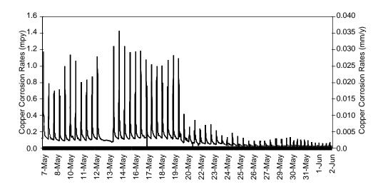
Figure 1: Improved corrosion rate results experienced with HRA under shot-feed chlorination. [TTA fed from May 7th until May 20th, equal actives of HRA fed for the rest of the time period.]
