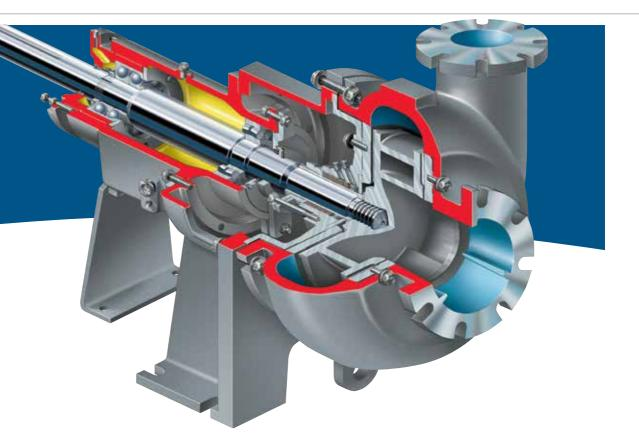
The Flowserve type M hard metal slurry pump is a horizontal, single-stage, end suction design with a tangential discharge nozzle. Fitted with a hard metal liquid end, the M pump is engineered to handle high concentrations of coarse, abrasive solids in suspension.
