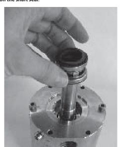
7. Scrap the old spacer (if black) and place the new white spacer on top of the retaining ball.
