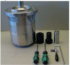
Unscrew the 4 mounting screws and remove the seal SAE flange. Do not yet unscrew the 2 lower screws.
