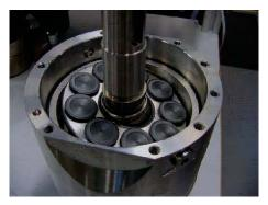
Use the plastic assembly tool provided, large diameter pointing downwards, to press the seal home against the shoulder of the spacer.
