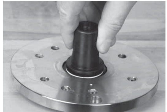
37. Press in place with special tool
