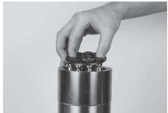
22. Mount pistons in housing
