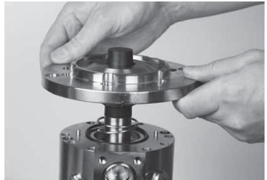
38. Mount flange on shaft (remember to spray with water)
