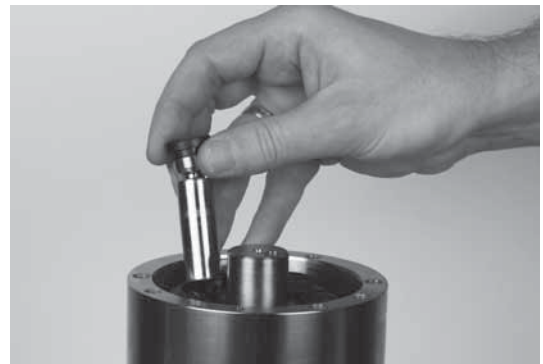
23. Mount the 2 last pistons
