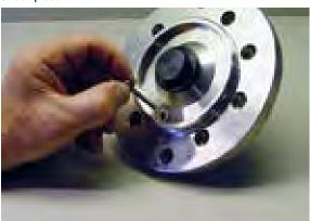
20. Tighten the screw to a torque of 5 Nm and remove the tool.
