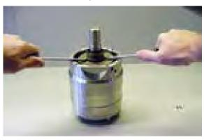
6. Remove the guide pin from the housing and the two guide pins from the swash plate.
