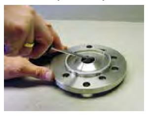
18. The ceramic ring removed from the front flange.
