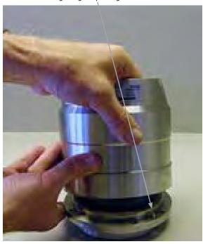
6. Mount the thrust plate with sealings on the cylinder barrel.
