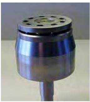
7. Press the thrust plate into the cylinder barrel using a table or the like as support.
