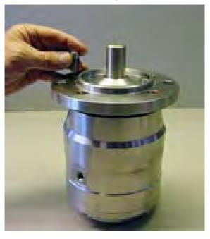
25. Tighten the screws to a torque of 30 Nm and mount the parallel key on the shaft.
