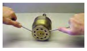
17. Remove the ceramic ring from the front flange.
