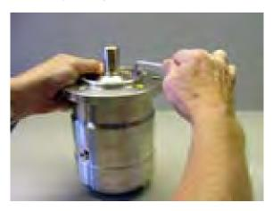
3. Unscrew the screws in the front flange.
