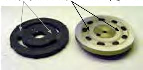
2. Hold a ruler against the surface of the plate and check the tightness against a light source.
