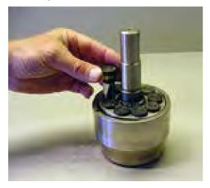
14. Remove the retaining plate.
