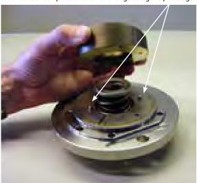
17. Press the swash plate against the flange andscrew the tools together.
