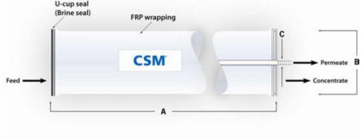
Each membrane elementsupplied with one brine seal, one interconnector (coupler) and four o-rings.
