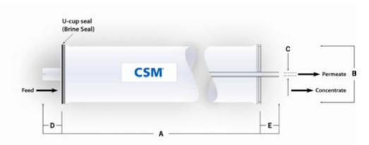
1. Each membrane elementsupplied with one brine seal, one interconnector (coupler) and four o-rings.
