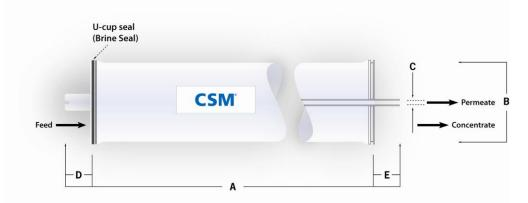
1. Each membrane element comes with one brine seal, one interconnector (coupler) and four o-rings. 2. All RE2521 elements fit nominal 2.5 inch (64 mm) I.D. pressure vessels.
