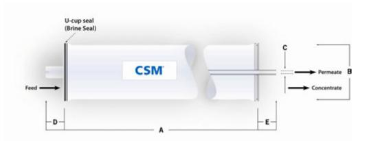
1. Each membrane element omes with one brine seal, one interconnector (coupler) and four o-rings.
