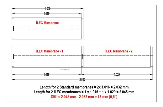
This fact will imply that in order to close the End caps of the pressure vessels, two types of End caps should necessarily be supplied:
