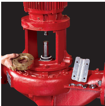
3) Disconnect seal flush line and remove gland plate bolts. The gland plate and seal seat may then be taken out between the shafts. With inside seal the complete seal is removed following the gland plate.
