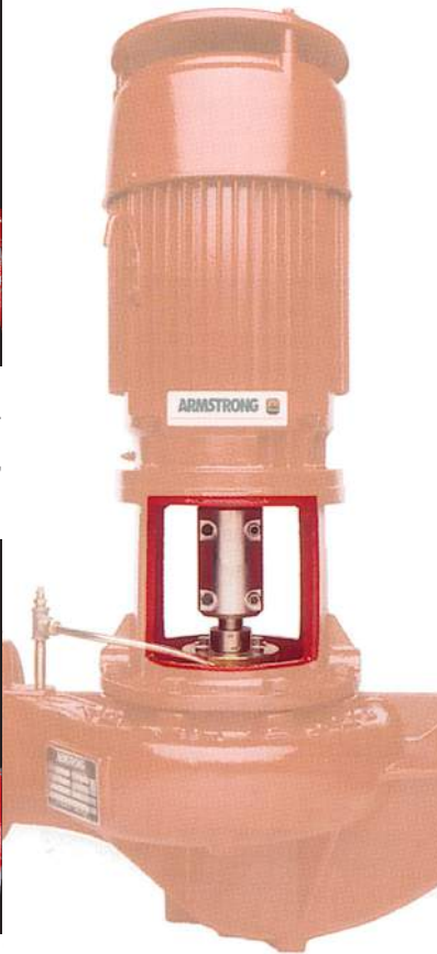
2) Remove the coupling bolts. The coupling halves (with drive and annular positioning keys) are taken from motor and pump shafts. Loosen set screws on seal rotating element and slide from pump shaft. (For inside seal see step 3)
