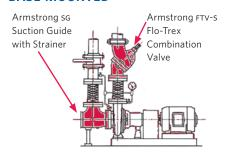
Base mounted pump with Suction Guide and Flo-Trex valve eliminates cost and space of:
