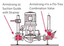
Vertical In-Line with Suction Guide and Flo-Trex valve eliminates cost and space of all the items listed under base mounted pump, plus the following:
