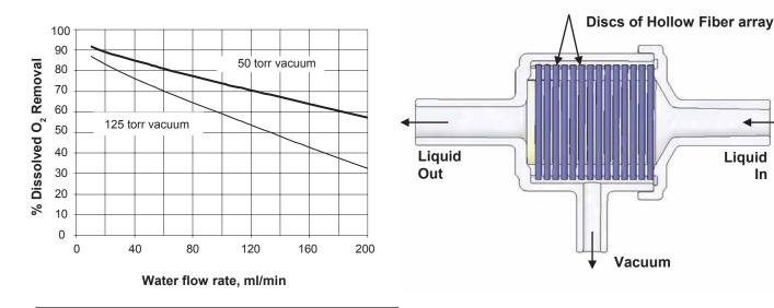
Curves represent nominal values generated using water on the shellside and vacuum on the lumenside at 20°C. Characteristics may change under different operating conditions.
