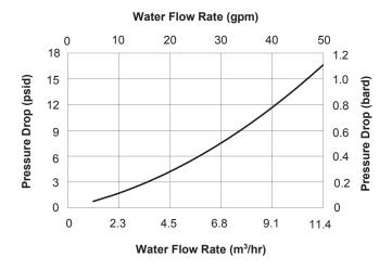
Curves represent nominal values using water at  $25^{\circ}$  C. Characteristics may change under different operating conditions.
