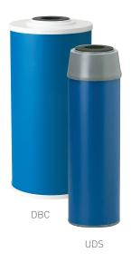
Pentair® Pentek® UDS & DBC series cartridges are enhanced with KDF media to inhibit scale buildup in the filter that can decrease product life. These cartridges are constructed of high performance granular activated coconut shell carbon and a 5-micron spun bonded polypropylene post sediment element for increased dirt holding capacity. They are effective for chlorine taste and odor reduction in high capacity situations and where lime and scale buildup problems occur.
