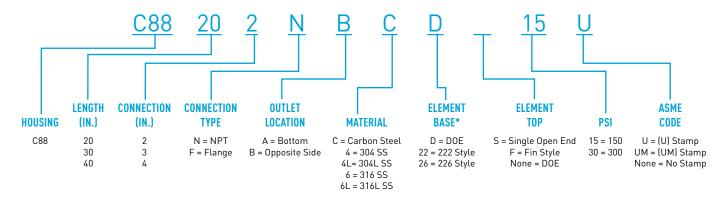
Note: If DOE, it is only required once in the part number and will specify both top and base. Cartridges are not included but must be specified as to the type using when ordering the housing. Carbon steel not recommended for water use as the epoxy coating is not designed as a corrosion inhibitor.
