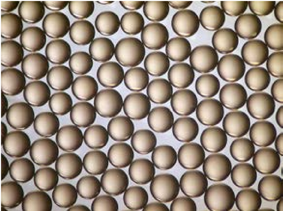
Figure 9: A gel-type Amberjet anion resin under the microscope
