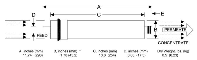
Core tube extension: E = 0.86" (21.8 mm)
