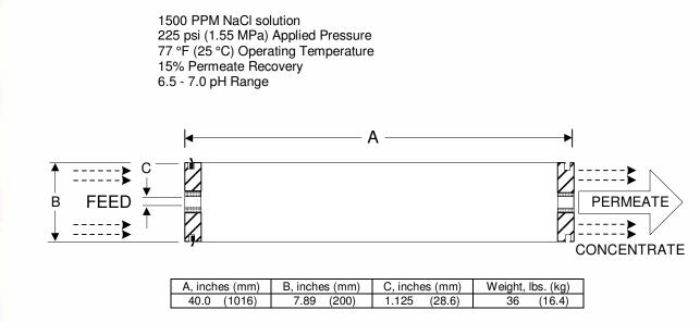
Notice: Permeate flow for individual elements may vary + 35 or - 15 percent. Membrane active area may vary +/-4%. All membrane elements are supplied with a brine seal, interconnector, and o-rings. Elements are vacuum sealed in a polyethylene bag containing less than 1.0% sodium meta-bisulfite solution and then packaged in a cardboard box.
