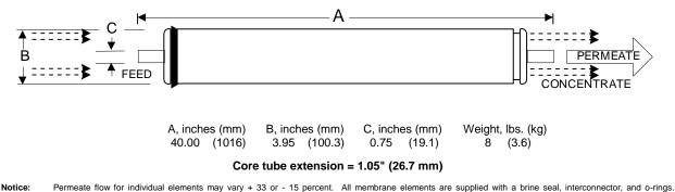
Nonce: Permeate now for individual elements may vary + 35 or - 15 percent. All memorane elements are supplied with a bine seal, interconnector, and o-imgs. Elements are enclosed in a sealed polyethylene bag containing less than 1.0% sodium meta-bisulfite solution and 10% propylene glycol, and then packaged in a cardboard box.
