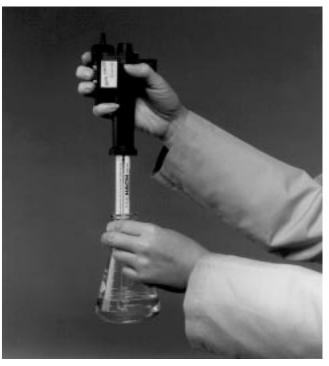
**4.** Immerse the tip of the delivery tube below the surface of the prepared sample and turn the delivery knob to begin titration. Continue titration until the end point is reached.
