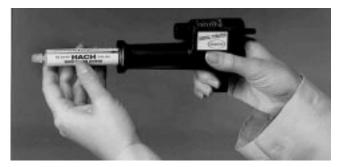
**2.** Remove the cap from the cartridge and install a delivery tube. Use a straight delivery tube for hand-held titrations or a 90° delivery tube for titrations using a laboratory stand to hold the titrator. Turn the delivery knob to flush the delivery tube with titrant and reset the counter to zero.
