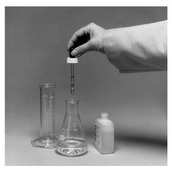
**3.** Measure a sample into a clean erlenmeyer flask and add buffers and/or indicators as required.
