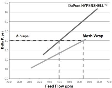
Pressure Drop versus Feed Flow for Mesh wrap and HYPERSHELL™ 8038 elements. HYPERSHELL™ has less exterior bypassing and requires approximately 30% less flow than mesh wrap for an equivalent pressure drop.
