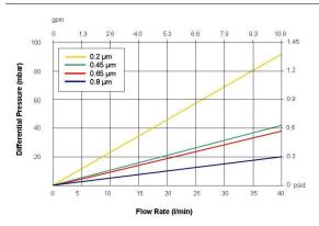
\*measured per 75 cm (30")element with water at  $20 \, ^{\circ}\text{C} \, 68 \, ^{\circ}\text{F})$
