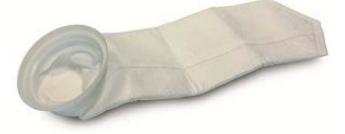
The no-bypass welded seams eliminate the possibility of fluid bypass through needle holes. We provide a variety of glazed and singed finishes to inhibit fiber migration. FSI also offers polyester inserted felts. These inserted felts include a reinforcing scrim needled inside the felt material, to provide added strength and durability, when a restrainer basket is not being used.
