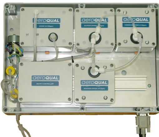
AQM 60 multi-gas sensor module with cover removed to show sampling pump, microcontroller module, four gas sensor modules plus temperature and humidity
