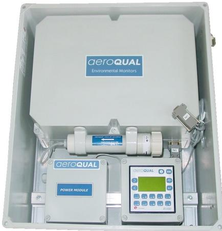
AQM 60 system installed in an external/outdoor enclosure and configured with multi-gas sensor module, zero-air scrubber, Programmable Logic Controller (PLC) and power supply module
