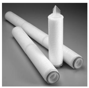
Aerex 2 0.2 µm hydrophobic cartridge filters provide high flow rates at low pressure differentials. Designed to remove bacteria and viruses from moist gas streams, the filters are ideally suited for use in industrial fermentation applications. Aerex 2 cartridge filters are manufactured using PTFE membrane and are 100 % integrity tested to assure optimal sterilizing performance. Each filter lot also must pass rigorous stress testing before release.
