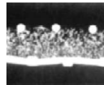
Figure 1: Cross-section of CUNO™ Super Metal Screen Filter Media
