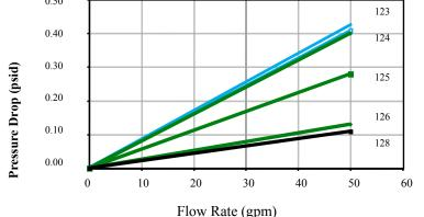
**Pressure Drop:** The 3M High Performance Filter Bags have low initial pressure drop ( $\Delta p$ ) in water as the chart indicates. The chart does include the pressure drop of a typical single vessel to assist you in sizing your filter system.
